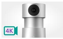
The camera shows speakers in remarkable clear 4k video with accurate color rendition. The 1/2.8 inch CMOS sensor ensures bright, clear video and sharpness even in low light settings.
