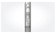
The quick-response and ergonomic slide switch is designed for singlehanded operation of all recording and playback functions, allowing easy and quick file editing (insert, overwrite, append). It operates with a light sensor signal, making it wear-free and durable.
